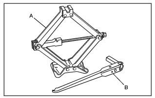
The tools you will be using include the jack (A) and the wheel wrench (B).
